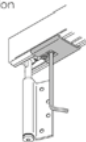
When cap screws loose, pivot arm can slide freely
